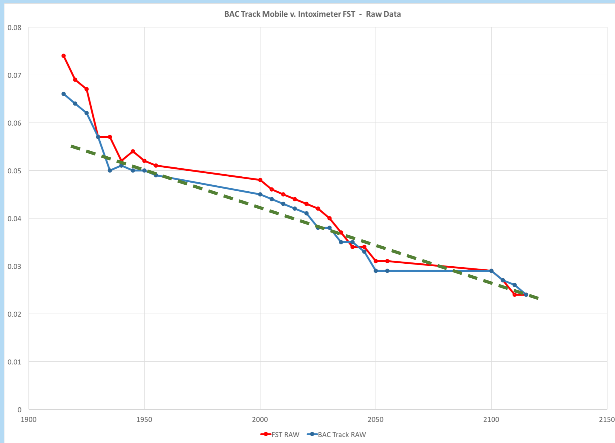
Figure 9 - Comparison of the Intoximeter FST (Red) with the BACtrack Mobile (blue). The overall downward trend is shown with the dashed green line.
